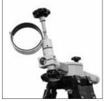
Furthermore, 33 cm adjustments are possible along the horizontal axis for precise alignment of the film focal spot distance.
